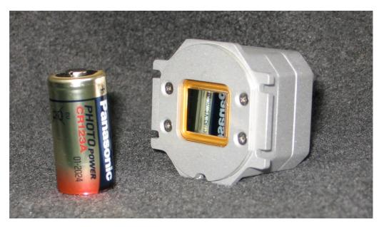
The Towcester Research TAPIR 640 camera engine provides a versatile compact low-cost and extremely rugged LWIR camera solution suitable for integration into a variety of platforms.
