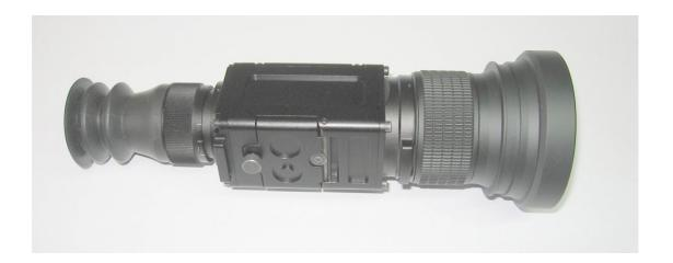
The Towcester Research SPIR 640-LR Long range Thermal Monocular operates in the Long Wave 8 to 12 micron IR band and uses the advanced shutterless TapIR thermal imaging engine containing the latest ULIS Gen2 640x480 pixel uncooled detector for maximum performance and exportability.
